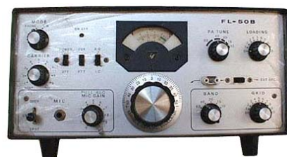
Sl. 39. Amaterski KT predajnik firme YAESU, model FL-50B
