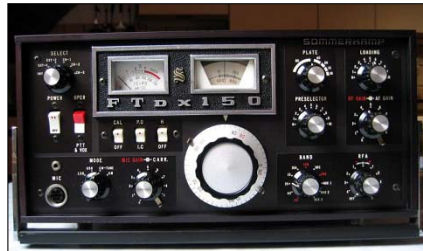
Sl. 34a. Prenosni transiver SOMERKAMP FTdx150
